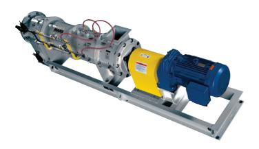
The material enters at one end of the cylinder and is whipped by the pins as it moves from the inlet through the shell and to the bottom outlets. As a fine spray of liquid is added at the entry section and distributed throughout the powder, fine mixing and micro-agglomeration will occur. The end result is a wetted, agglomerated and densified micro-pellet.
