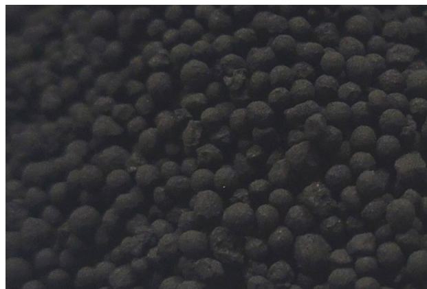
Representative rCB pellets used in laboratory and pilot-scale evaluation of pellet hardness, flowability, and dispersion
